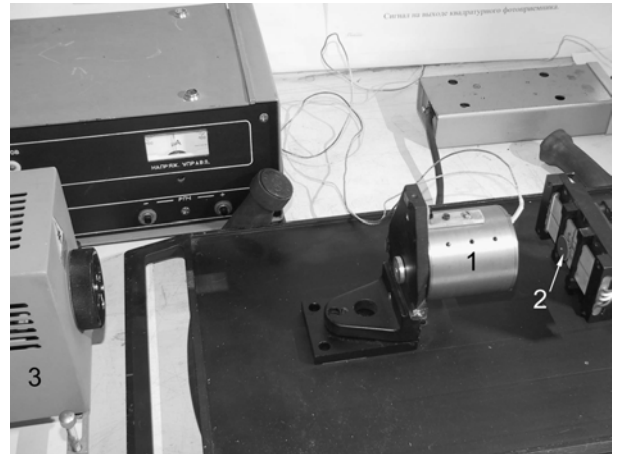
Fig.6. The scheme of an one-reflecting interferometer. Here: 1 - photodetector responsive to an interference field; 2 - mirror; 3 - light source; 4 - collimator.
